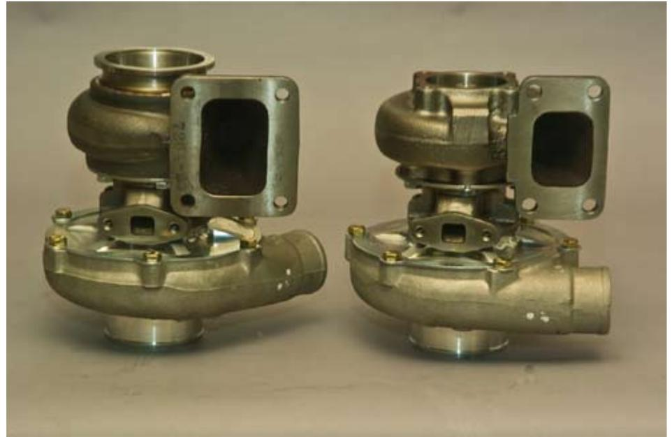
Above: note the size difference of the two hot sections and two cold sections. A turbo is not just a turbo ... it is built to specifications for the intended purpose.
