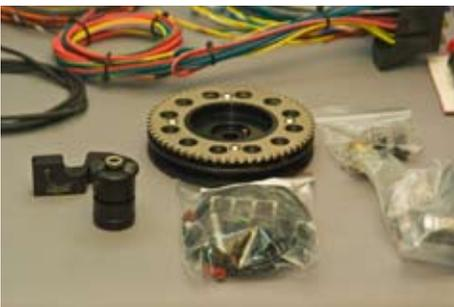
Above: a visual feast ... crank timing wheel, distributor hole plug, harness, etc.
