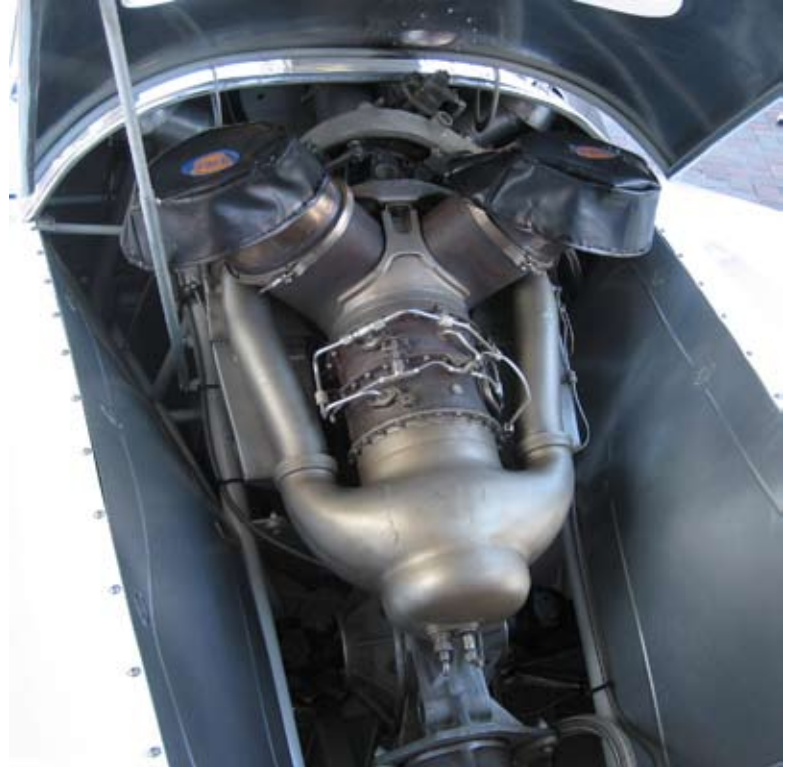
The Howmet TX with Allison turbine. Small, hot, a lot of torque. A lot of potential ... perhaps. Photo by "The 359"
