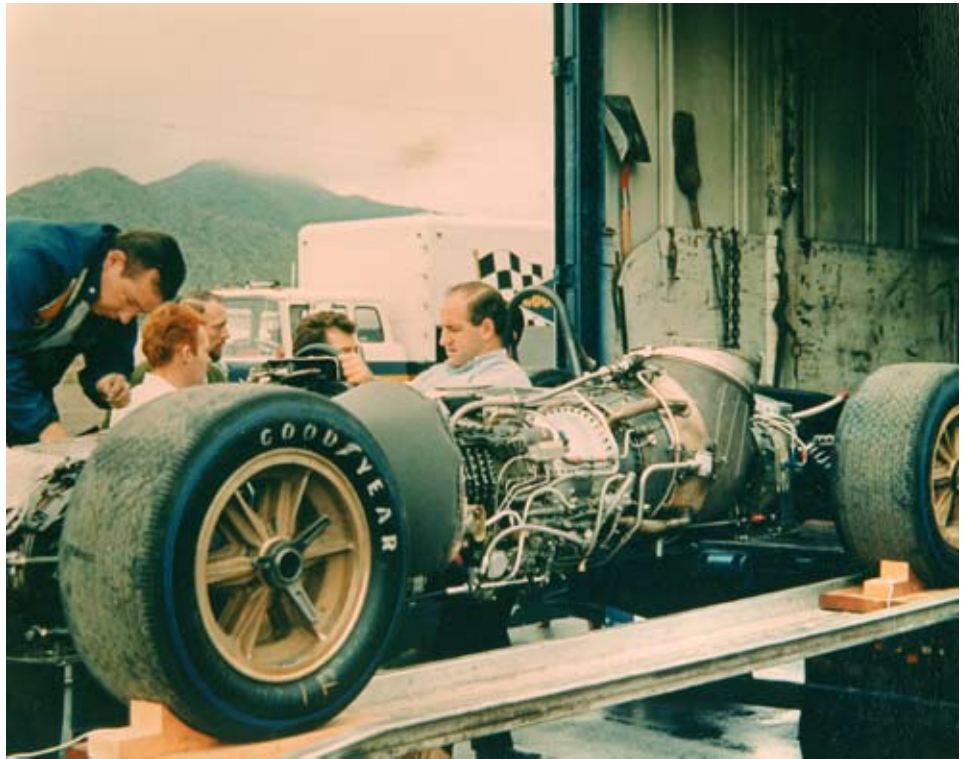
An Indy 500 car of the 1960s with a T-58 turbine installed. Photographer unknown.
