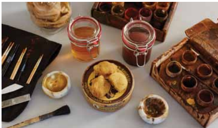
The tools of Rob's trade include shellac crystals with alcohol, mentholated spirit-based varnish, and boxes containing aniline dyes, from which he makes stains
