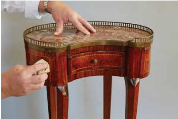
Photographed by Greg West Hanna demonstrates the technique of French polishing, which provides a high luster
